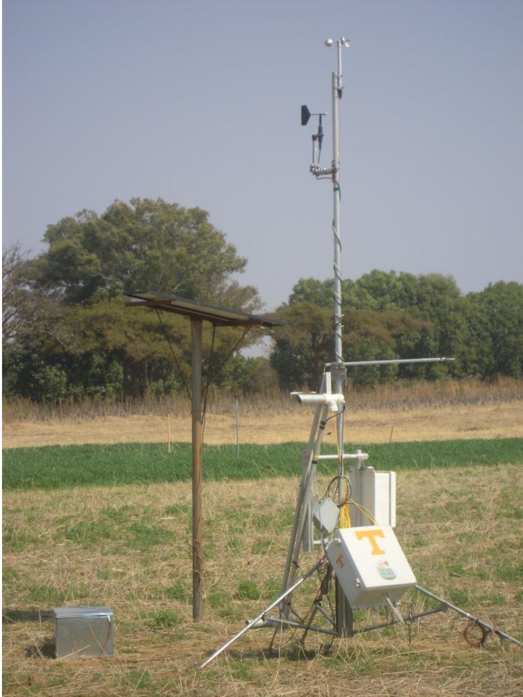
Figure 8 Micrometeorological station with rotating arms at the Mt. Pleasant, Zimbabwe study site
